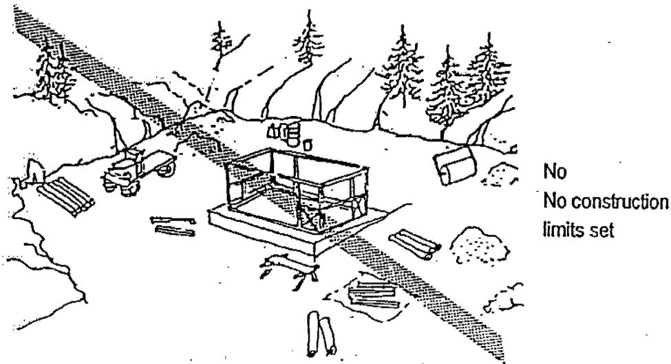
Measure must be taken to identify the area of disturbance in site, tag all trees over 6" in diameter within the area of disturbance and provide construction limits through the use of stakes and ribbon. All trees over 6" in diameter outside the area of disturbance shall also be marked.
